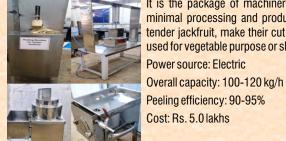
It is the package of machinery for processing of tender stage jackfruit for minimal processing and production of powder. It includes peeling of whole tender jackfruit, make their cut pieces, anti-browning treatment which can be used for vegetable purpose or shredded, dried and converted into powder.
